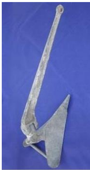
Figure A-4 articulated plough anchor [4]
