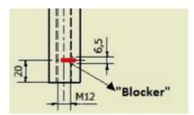
Figure 6-7 Method of locking the eye bolt
