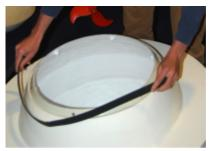
Figure 6-14 EPDM rubber tape (3mmx25mm)
