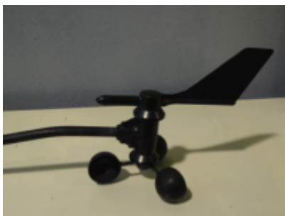
Figure 6-31 Weather vane is turned 0° → 0V
