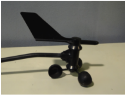
Figure 6-32 Weather vane is turned 180° → 1,65V
