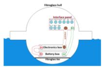
Figure 6-28 Waterproof connections inside the hull
