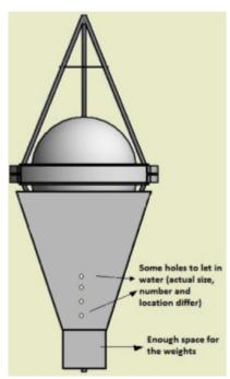
Figure 7-2 Fibreglass cover
