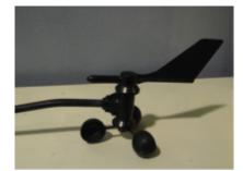
Figure 6-31 Weather vane is turned 0° → 0V
