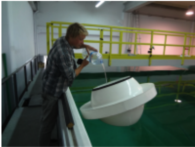
Figure 6-34 Test for buoyancy of the fiberglass hull
