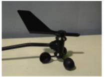
Figure 6-32 Weather vane is turned 180° → 1,65V
