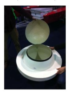
Figure 4-8 The fibreglass hull
