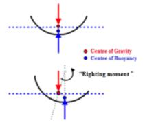
Figure 6-10 Centre of gravity and centre of buoyancy
